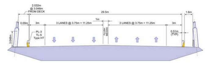
Proposed Bridge Typical Cross Section<sup>b</sup>
